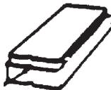
USE AN IC PULLER OR A SMALL SCREWDRIVER TO REMOVE THE EPROM
